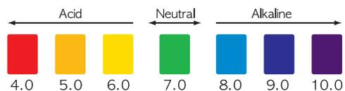
How to Measure: Place 10-15 mL of test water in a container and add 2-3 drops of reagent. Then mix well and check the color of the water with the pH chart above. (The color depends on water quality and reagent.)
